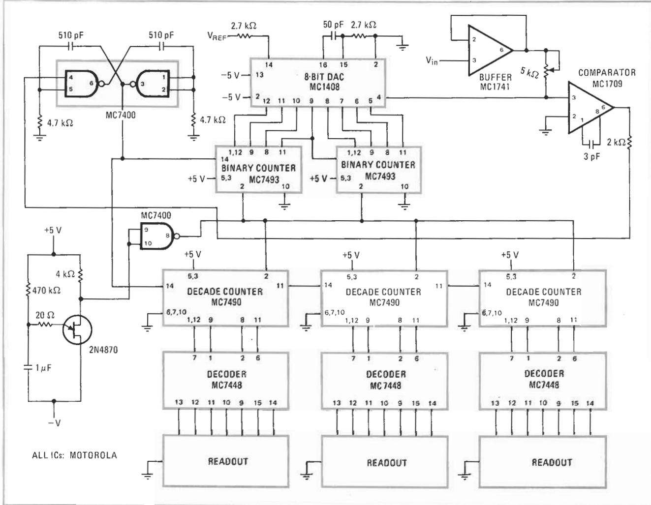
**DVM details.** Unknown input signal is compared to the output current from the digital-to-analog converter. When these two signals are equal, the clock is stopped. The same clock is used to drive the converter's binary counters and the display's BCD counters.
